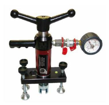
The extractometer is a portable system allowing you to test anchors.
